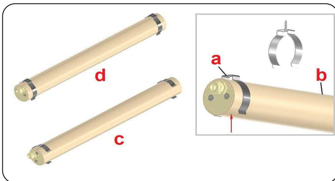
**STEP 5 :** A second system consists of a T-shaped plate (a) and a tensioning strap (b), which are connected to each other with a bolt, knurled washer and a nut. The rubber on the tension strap will provide the grip on the Plexiglas cylinder. The T-plate has two mounting holes for chipboard screws (c).
