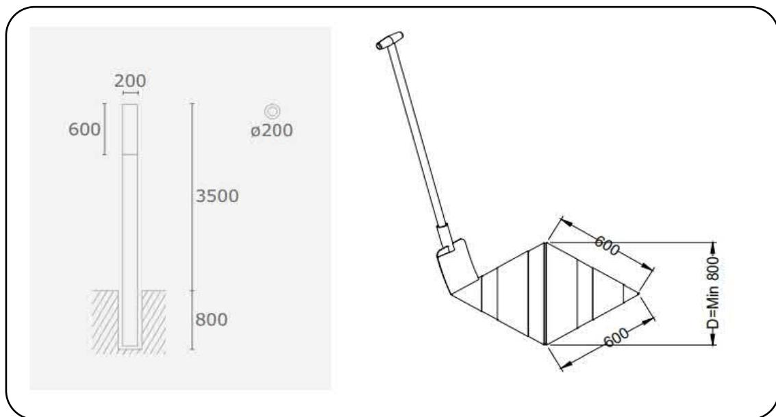
**STEP 2 :** Run the supply cable through the bottom of the luminaire (a). Place the pole in the hole until the door of the luminaire is located 600 mm above ground level (b) and fill up the hole with stabilized sand or a concrete mixture. Make sure that the pole is standing upright (c).
