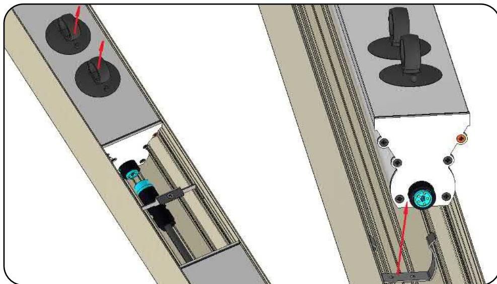
**STEP 1.3 :** Transfer the dimensions of the slotted holes to the ceiling. Also keep in mind the power point. A larger opening has been milled for passage of the power cable. Drill the mounting holes in the ceiling and secure the profile with chipboard screws.
