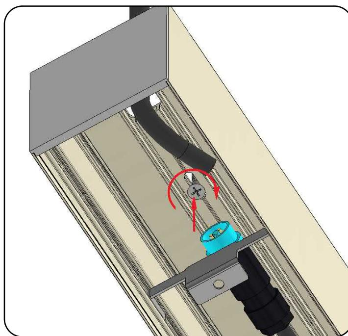
**STEP 1.4 :** Insert the power cable. Remove the outer sheath (b) from the cable and strip the wiring. Slide the cap with cable gland onto the cable, insert the wires into the terminals of the mating plug (a) in the correct position and screw tight. Slide the cover towards the socket until it clicks and tighten the gland. Connection data is included. Turn the plug and socket against each other until they slide into each other. Press until there is a click. Both plugs are locked together.
