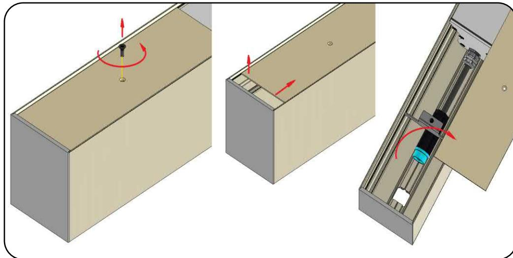
**STEP 1.2 :** If necessary, remove the light profile with the supplied suction cups. Place the suction cups on one side next to each other and push the air from underneath so that they adhere well. Then pull the light profile out of the basic profile. All mounting holes are now accessible from the inside.
