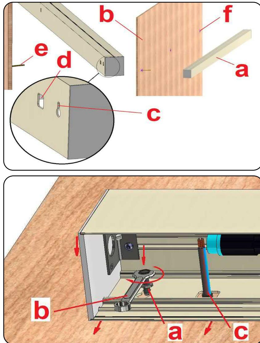
**STEP 3.2 :** Connect the female connector to the power cable in the ceiling as mentioned in step 1.4. Insert the female plug into the plug until it clicks. The plugs are now locked. The shield can be moved or pressed back into the profile.
