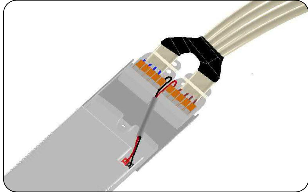
**STEP 1.2b :** When using a single R20 fixture on a LED driver, connect the cable directly to the red and black terminal of the LED driver itself with the color code as stated in step 2.1. Use the strain relief on the LED driver module to clamp the wire.
