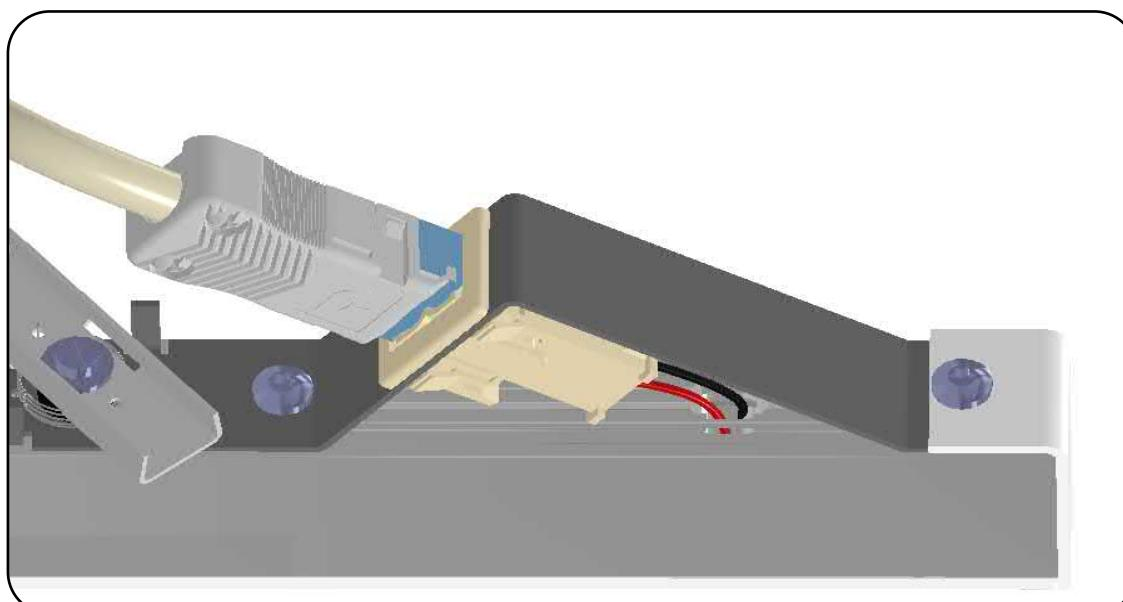
**STEP 1.4 :** To remove the plug (b) from the socket (a), you need a fine flat screwdriver (c) of 2.5 mm width. Insert the screwdriver into the opening (f) between the plug and the socket, up to the slot (d). Moving the screwdriver down on the edge of the housing and pulling the plug(e) will release it.
