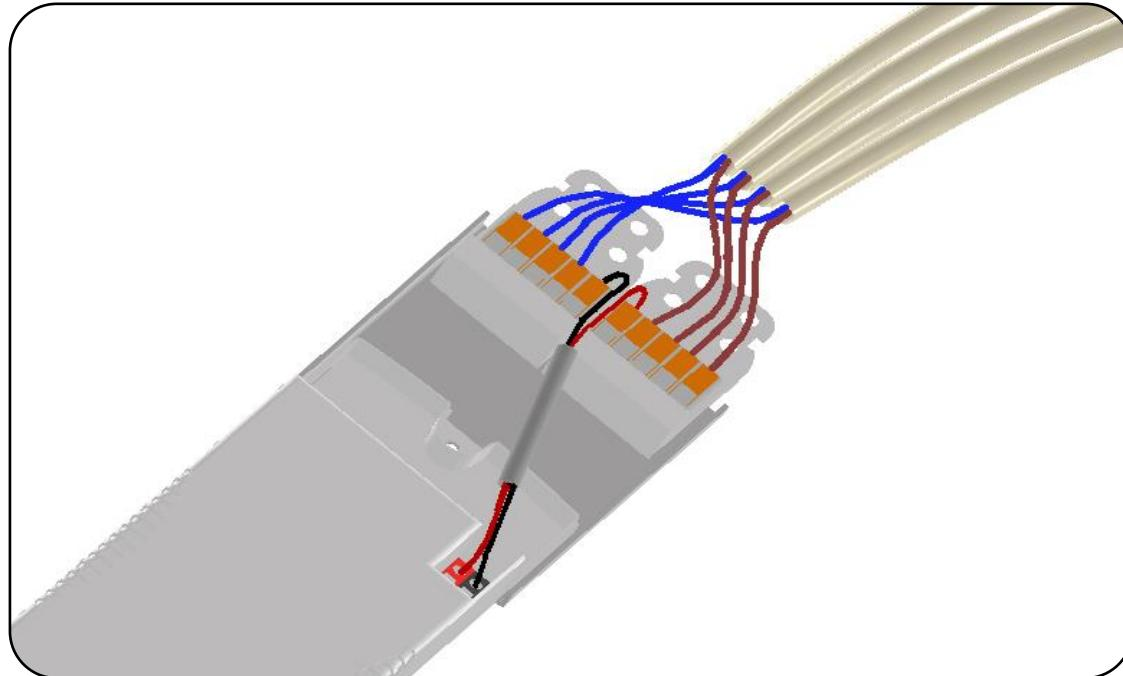
**STEP 3 :** Insert the plug on the fixture into the provided socket.
