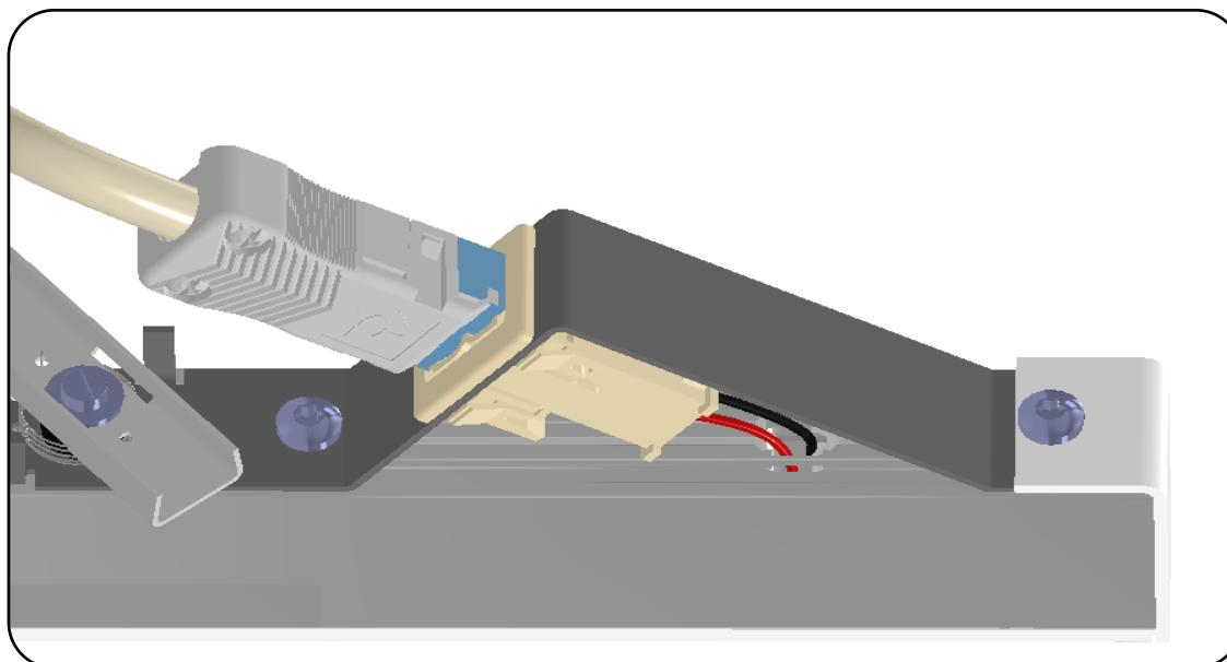
**STEP 4 :** To remove the plug (b) from the socket (a), you need a fine flat screwdriver (c) of 2.5 mm width. Insert the screwdriver into the opening (f) between the plug and the socket, up to the slot (d). Moving the screwdriver down on the edge of the housing and pulling the plug(e) will release it.
