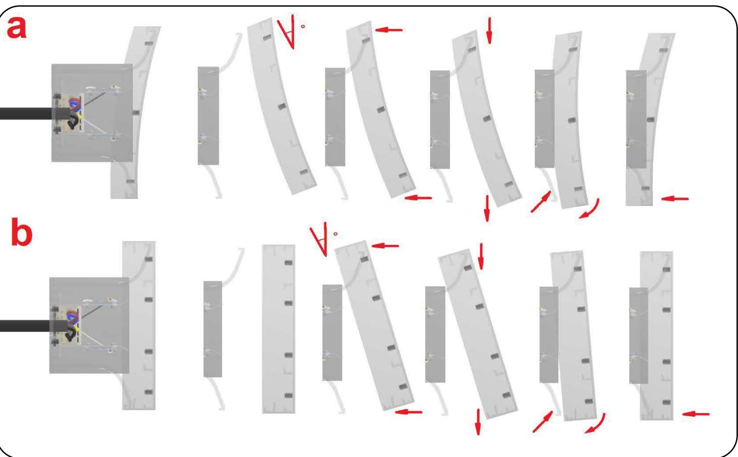
**STEP 5 :** Profiles of the T-Line 130 (a) are coupled with a coupling plate (b), which is already fixed on one side with set screws. Slide both profiles well against each other and tighten the remaining set screws as well. The cover is placed, slightly offset from the coupling seam. The electrical connection is made by connecting the wires from one fixture to the terminal of the next fixture.
