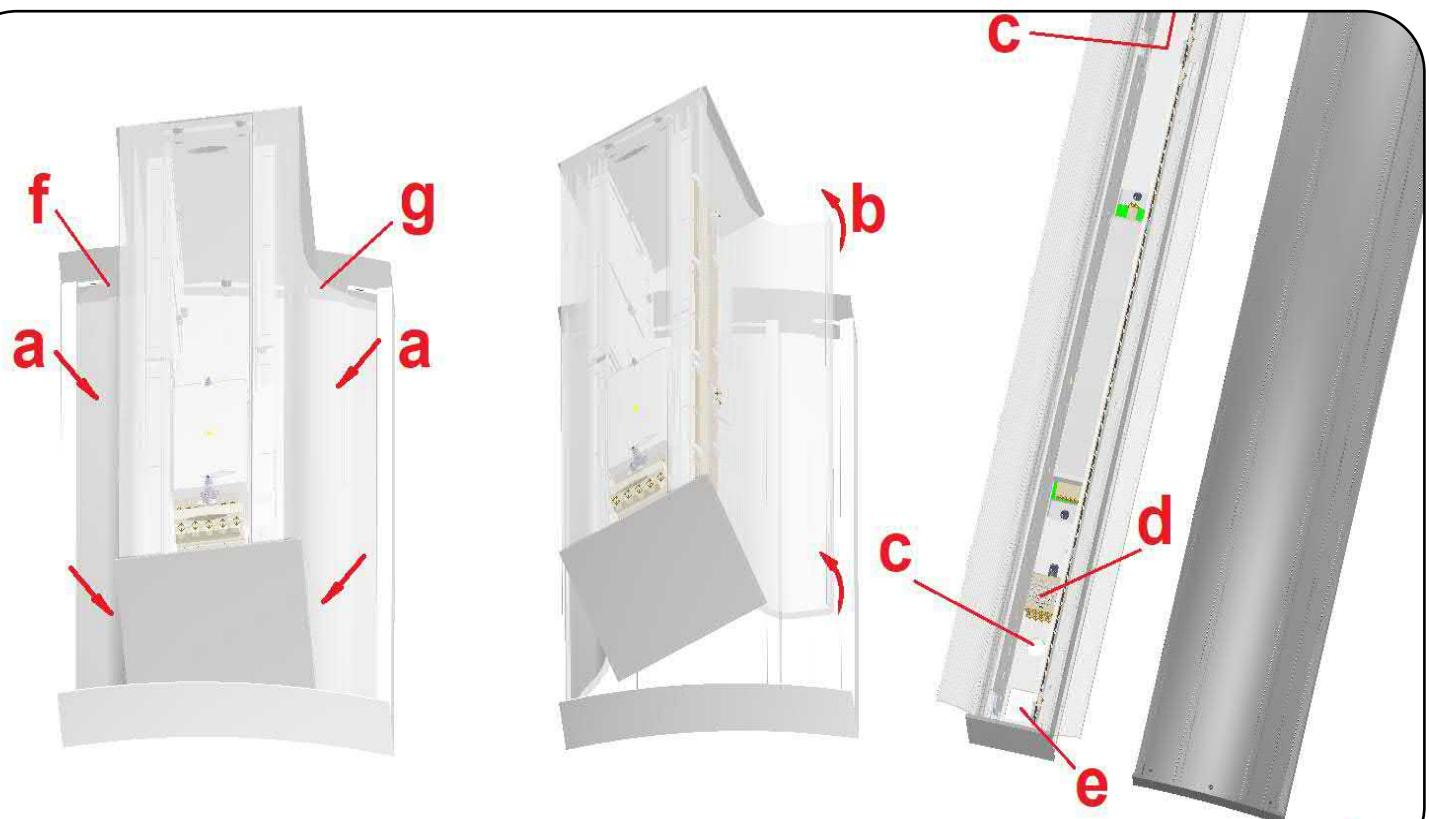
**STEP 2 :** Included is an oval disc with perforations (a). Slide this over the mounting hole and insert the chipboard (c) through the hole (b) and tighten gently. By moving the plate (d) in the slots (e), the luminaire moves upwards or downwards. This makes it possible to align or level the fixture. Once in position, tighten the screw further.
