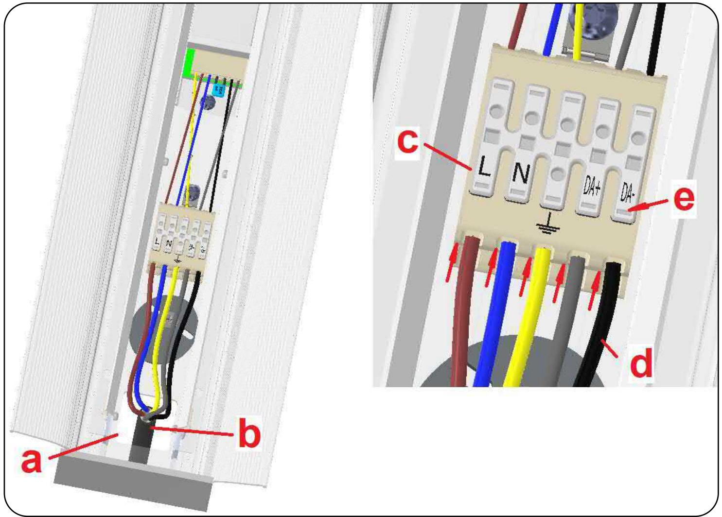
**STEP 4 :** Place the cover back. Depending on the type chosen, the luminaire has a curved cover (a) or a straight cover (b). Hold the cover with the opening to the fixture at an angle. Slide it over the top wide diffuser side and lower it. Bring the cover at the bottom towards the lower narrow diffuser side, lift the diffuser side slightly and press the cover over it.
