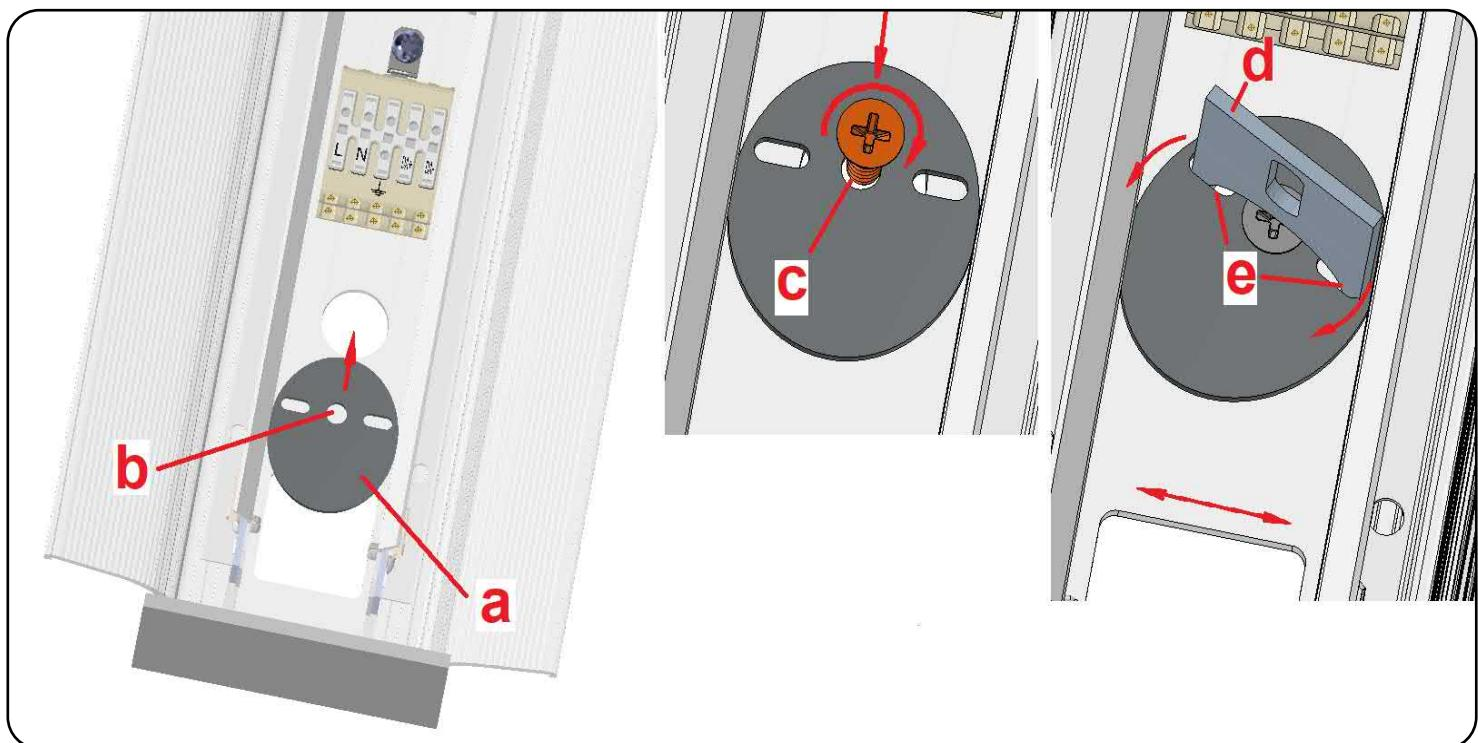
**STEP 3 :** Use the square opening (a) to insert the power cable (b). Dismantle the 10 cm cable and strip the 9 mm wires. The delivery includes a diagram with the colour code of the wires and the connection to the terminals (c). Insert the stripped wire (d) into the terminal. The wire can be accidentally removed from the clamp by lightly pressing the clip on the clamp (e) and pulling the wire.
