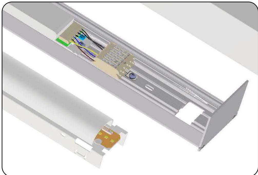
**STEP 1.4 :** Fasten the luminaire with chipboard screws (a) and possibly a washer (b). Insert and dismantle the power supply cable (c). Strip the wires (d) and connect them to the terminals (e) according to the supplied color code. Bend the wires (f) coming from the LED driver in a position to connect.
