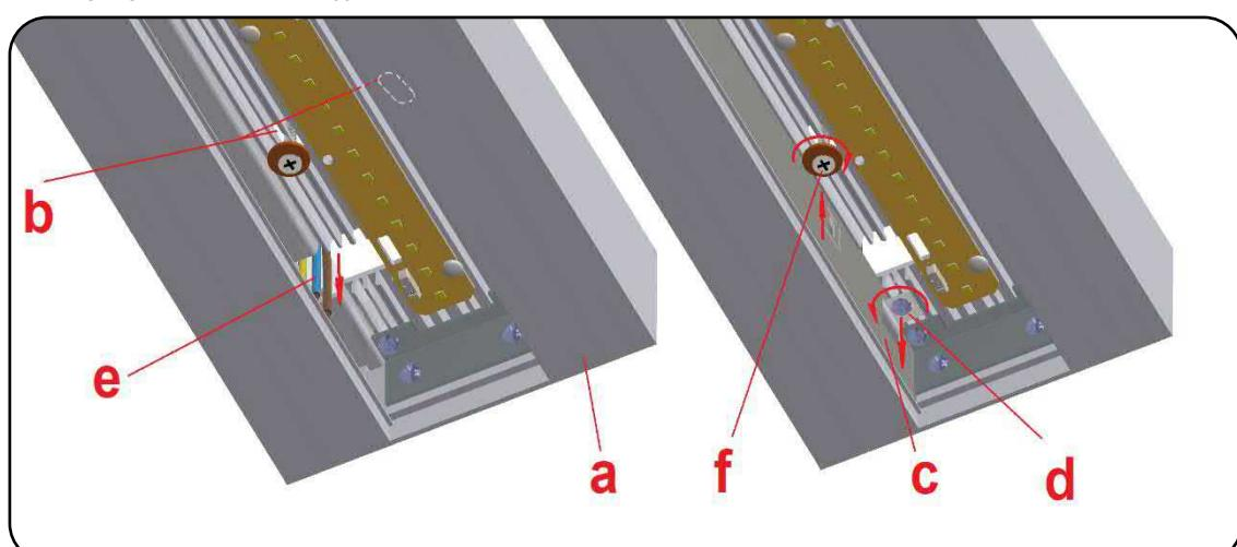
**STEP 1.3 :** Slide the side reflector (a) at the rectangular cable entry to the center of the profile. The mounting plate with LED driver (b) will now appear. Connect the wires (c) to the terminals (d), according to the supplied connection data. Then slide the side reflector back into place and screw tight.
