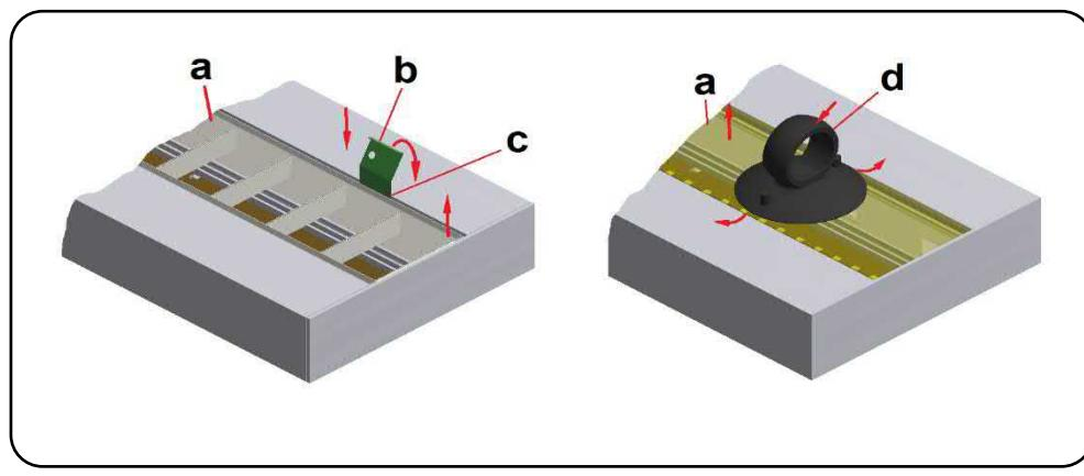
**STEP 1.2 :** Copy the dimensions of the slotted holes (b) from the base profile (a) on the ceiling. At the position of the supply, it is also necessary to unscrew the bolts (d) of the side reflector (c) and remove the side reflector. Enter the power cable (e) through the rectangular cable gland and leave the cable at its length. Screw the base profile to the ceiling with chipboard screws (f).
