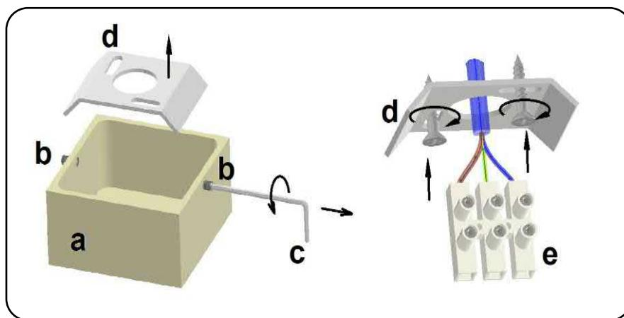
**STEP 2.2 :** Connect the cable of the luminaire to this terminals (a). De-duplicate the grounding (d) and fasten it to the grounding tab (b) in the base. Then fit the cable with the supplied strain relief (c) and tighten it firmly. Bring the canopy over the mounting plate and tighten with the set screws. Optionally, the cable can be attached to the steel wire of the suspension with the small cable ties.
