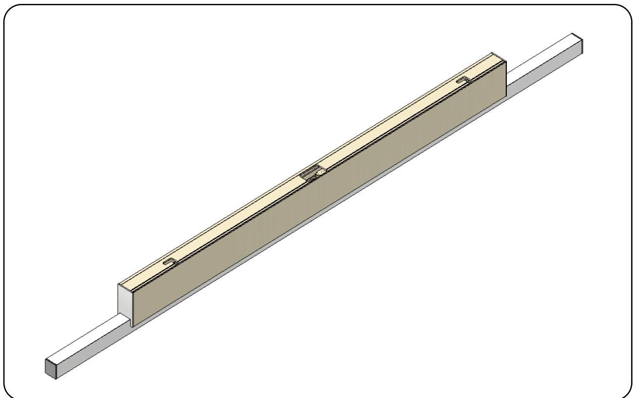
**STEP 2.2 :** Measure the distance between the 2 ends of the milled slotted holes and mark these holes (a) in line with the feed point (b). Drill the holes and preferably screw in a threaded bolt (c) with a hexagonal head. Let the head protrude a few millimeters from the wall.
