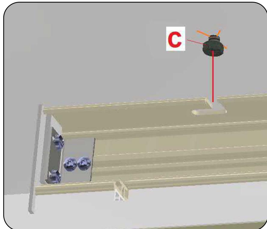
**STEP 2.3 :** Slide the profile with the milled recesses over the threaded bolts to the end. Also pull the power cable to length in the profile.
