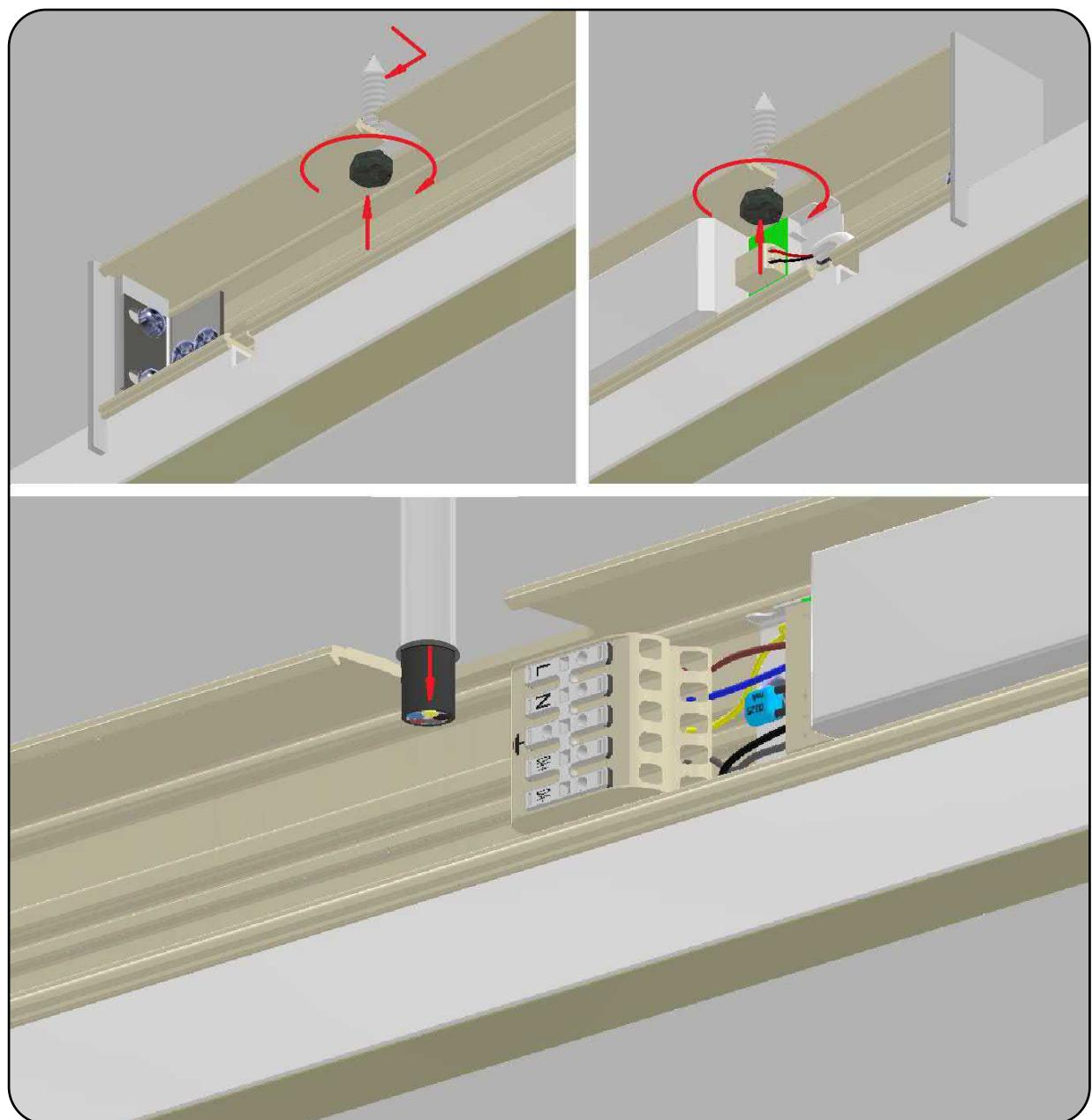
**STEP 2.4 :** Dismantle the power cable (a) and strip the wire ends about 9mm. Slide the profile laterally over the threaded bolts and lower the profile (b). Tighten the threaded bolts with a wrench (c). Insert the wire ends into the terminals according to the supplied connection diagram. Hook the side wall (e) into the back of the base profile and press the front of the side wall towards the light profile in the base profile until you hear a click (f).
