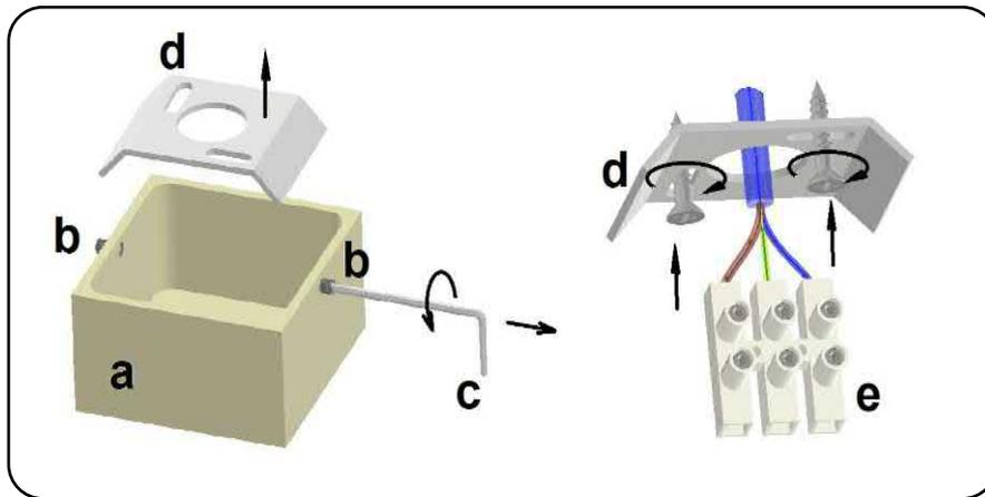
**STEP 2.2 :** Connect the cable of the luminaire to this terminals (a). De-duplicate the grounding (d) and fasten it to the grounding tab (b) in the base. Then fit the cable with the supplied strain relief (c) and tighten it firmly. Bring the canopy over the mounting plate and tighten with the set screws. Optionally, the cable can be attached to the steel wire of the suspension with the small cable ties.
