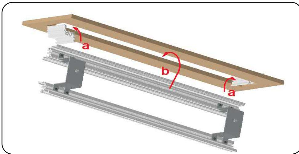
**STEP 3.4 :** Insert the supplied template into the gap between the profiles to mark the mounting holes. Make sure that the finishing profiles fit against the mold, this is the luminaire width + 1mm. The number and distribution of the holes depends on the length of the fixture, we recommend every half meter. Drill the holes and fasten the profiles with countersunk screws.
