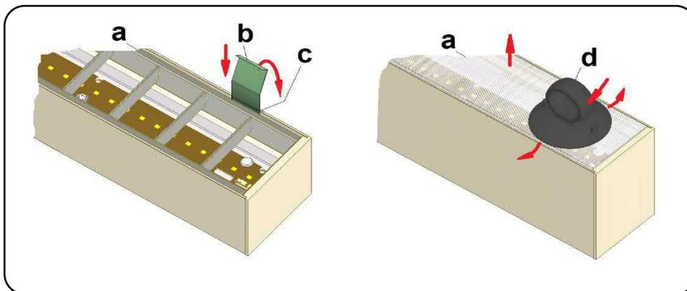
**STEP 1.2 :** The R65 profile has slots on the rear wall for screw mounting. These are accessible by removing the inserts with LED boards, which are already electrically disconnected, where the screw mounting is. You can also disconnect the wires yourself by pressing the release tool (a) into the opening of the terminal (b) and pulling the wire. If there are several inserts, disconnect the intermediate connection (c).
