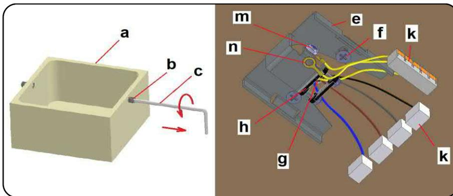
**STEP 2.1 :** Pull the connection cable (a) of the fixture through the opening in the cover and clamp them into the strain relief (b). Insert the wires (c) according to color into the terminals (d). Make sure that the cover is connected to the earth (e). Insert the terminals on the side into the cover (f), slide the cover over the base plate so that the adjusting screw (h) fits over the sloping piece (g) and tighten both adjusting screws with the Allen key.
