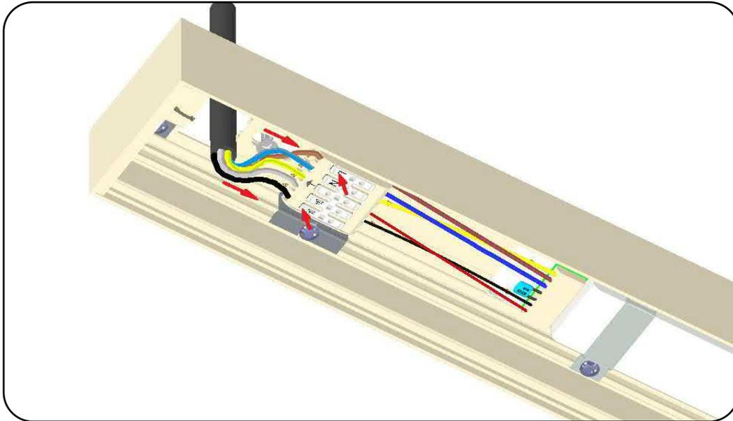
**STEP 1.6 :** Press the insert (a) with LED boards back into the base profile (b). Plug the wiring from the LED driver back into the terminal on the LED board. ( c ) ( white = + ) ( grey = - ).
