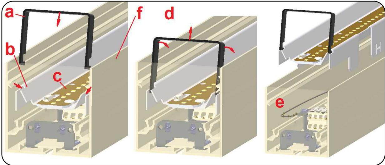
**STEP 1.4 :** Copy the dimensions of the slotted holes on the ceiling. Also keep in mind the power point. A larger opening has been milled for passage of the power cable. Drill the mounting holes in the ceiling and secure the profile with screws (b) that are sufficiently strong to support the weight of the luminaire.
