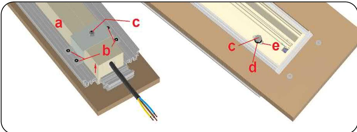
**STEP 3.3 :** Insert the short finishing profiles (a) at the narrow ends above the ceiling. Pay attention to the way in which the supporting structure is put together (12 or 15 mm side). Insert the long finishing profiles with screwed mounting brackets with a rolling movement (b) on the ceiling and lower the structure into the opening. Also pull the short finishing profiles down into the opening, so that the whole forms a frame.
