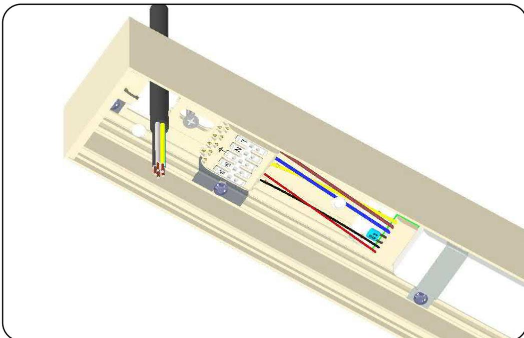
**STEP 1.5 :** Insert the power cable. Remove the outer sheath from the cable and strip the wiring about 9mm. Then insert the wires into the terminal in the correct position. Connection data is included.
