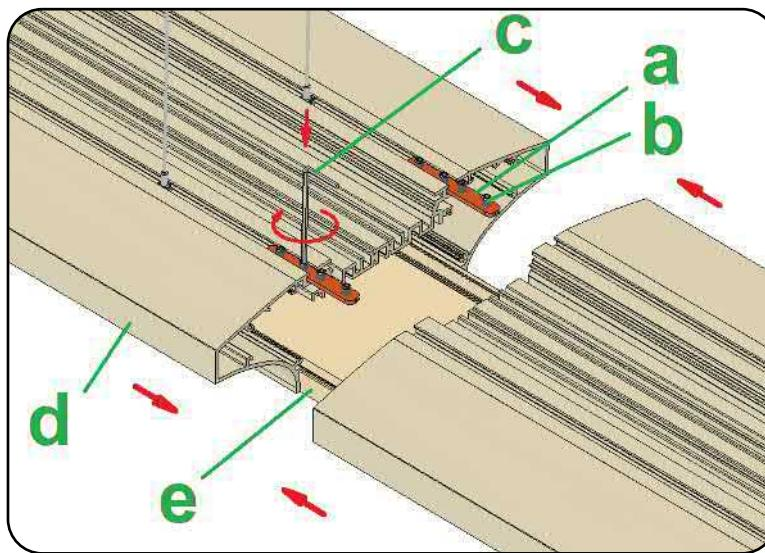
**STEP 1.5 :** Finish the seam (a), which occurs when 2 profiles are joined, with the supplied silicone sealant (c). Use tape to stick on both sides of the seam(b). Press the contents of the syringe(c) into the joint(d). Rub the sealant with a damp cloth to get the smoothest possible result. Remove the tape and a tight joint(f) will remain on the seam.
