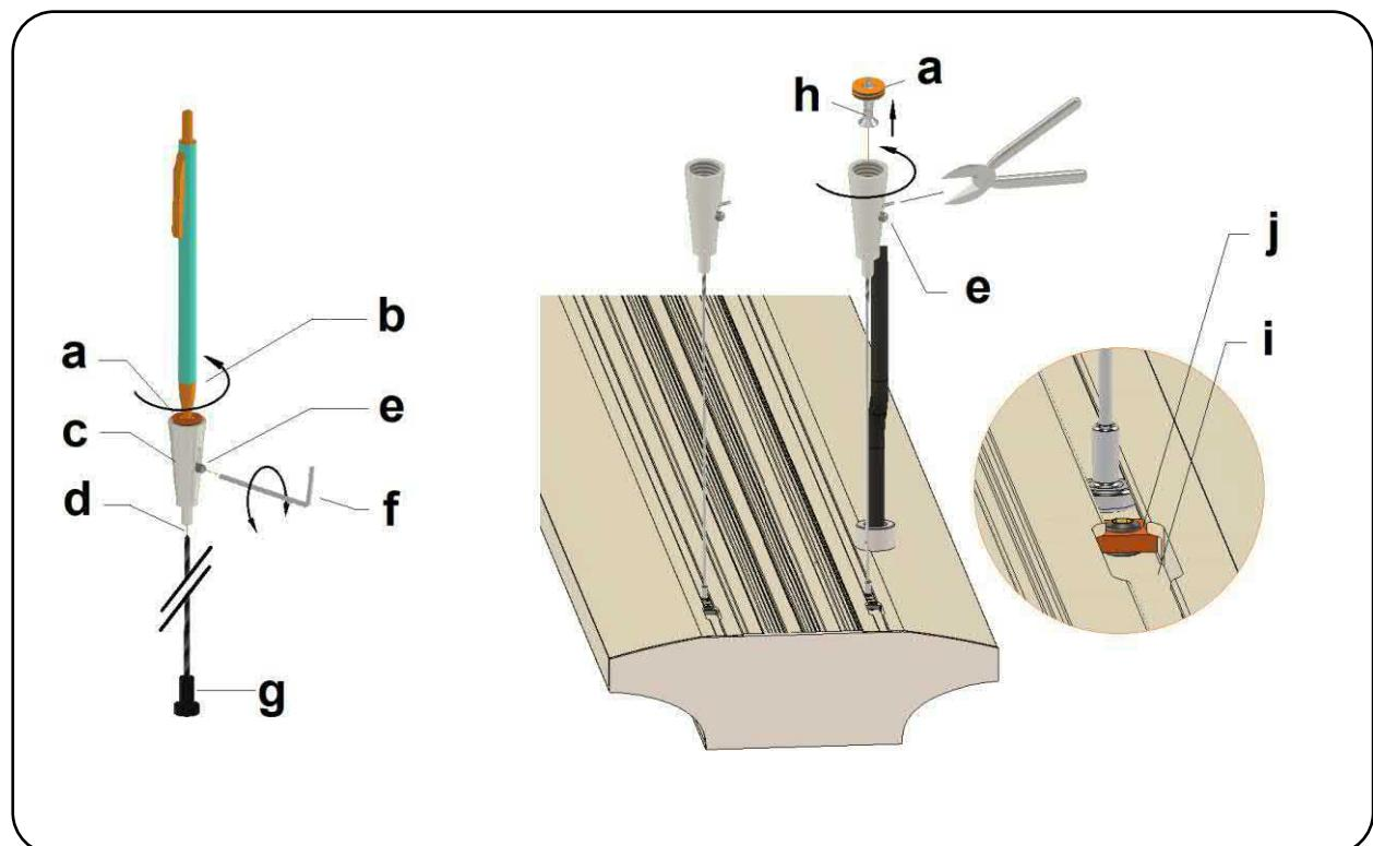
**STEP 1.4 :** Two coupling plates (a) are used to connect two profiles. One side of the profile is then already provided with the coupling plates, secured with set screws (b). Press both profiles (d) well against each other to obtain the finest possible seam and allow the coupling plates to slide into the suspension channel. Tighten the remaining set screws with the Allen key (c). Replace the shield (e).
